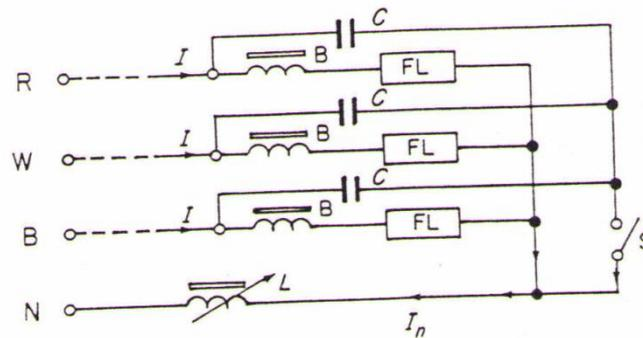
Figure 5 Three-phase fluorescent lighting test circuit. FL, fluorescent lamp; B, ballast; C, power factor correction capacitor; L, variable inductor; S, switch to isolate capacitor star point.
