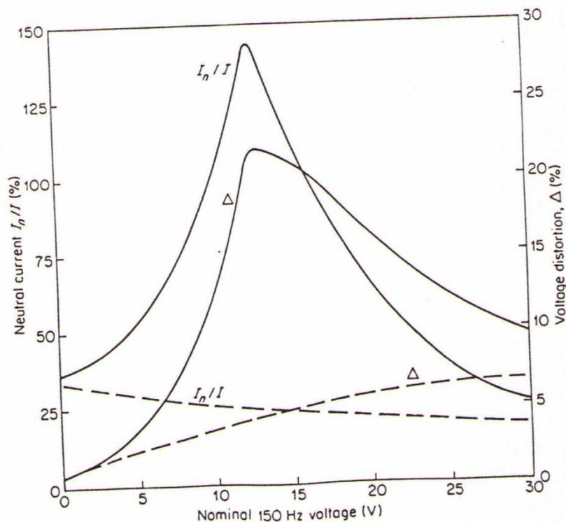
Figure 6 Characteristics of the fluorescent lighting test circuit. The nominal 150 Hz voltage is the calculated product of the 150 Hz lamp current per phase and the circuit zero-sequence impedance (150 Hz). —, Switch S closed (star point to neutral); ----, switch S open (star point floating)
