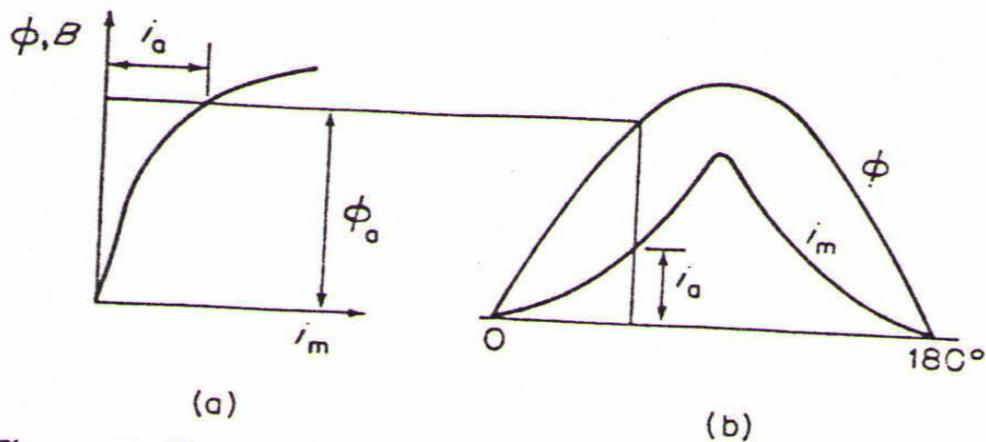
Figure 6 Transformer magnetization (without hysteresis): (a) magnetization curve; (b) flux and magnetization current waveforms
