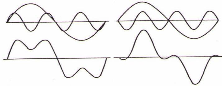
FIG. 1 Effect of harmonic phase angle on waveshape.
