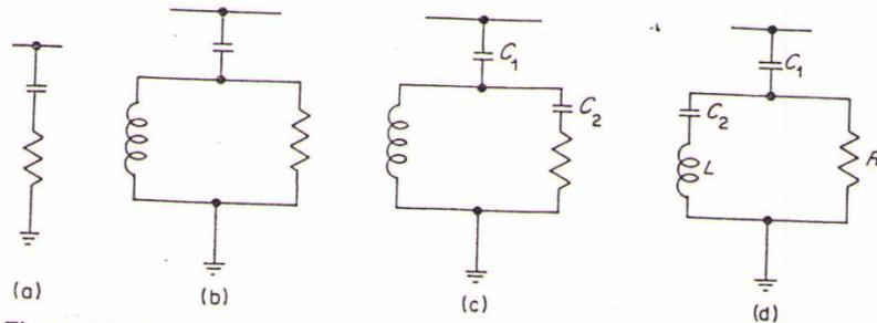
Figure 10.7. High-pass damped filters: (a) first order; (b) second order; (c) third order; (d) C-type
