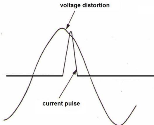
FIG.2 Current pulse from television receiver with thyristor power supply and consequent voltage distortion
