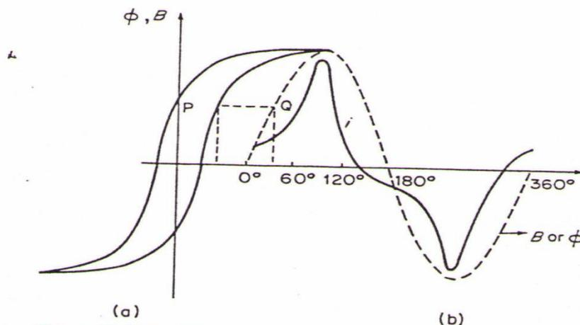
Figure 4.2. Transformer magnetization (including hysteresis): (a) magnetization curve; (b) flux and magnetization current waveforms
